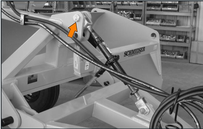
2. Flip pull frame up to rest between top clevis ears.
